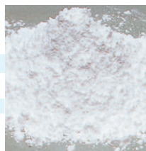
Calcium carbonate+fatty acids (surface modification)
